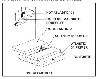
Note: Any Atlas Mortar Powder can be sprinkled over the finished surface to prevent sticking to workmen's shoes or boards which have been laid down as walkways. If powder is used between layers, sweep it up before applying the next layer or the layers will not adhere to each other. NO TRAFFIC OR EQUIPMENT SHOULD BE ALLOWED ON THE MEMBRANE UNTIL THE BRICK SHEATHING, WHICH IS ALWAYS REQUIRED, IS INSTALLED.
