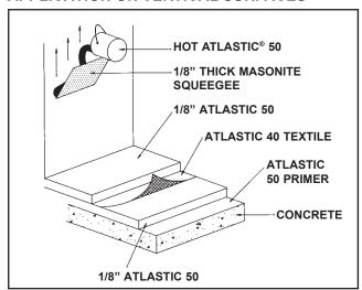
g. If a 3/8" (9.5 mm.) thick ATLASTIC 50 MEMBRANE is desired, apply as described above, however, place 3/16" (4.8 mm.) thick layers of ATLASTIC 50 instead of 1/8" (3.2 mm.).
