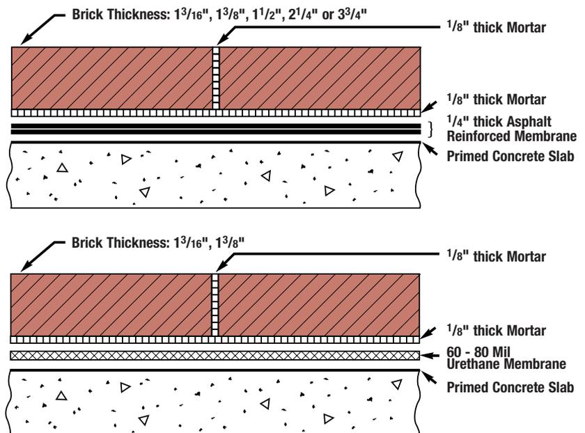
**Heavy Duty** — 2<sup>1</sup>/<sub>4</sub>-inch thick single brick for heavy trucking and extremely wet operations.
